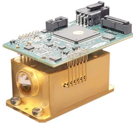
Figure 2: An example of a modern day QCL tuner produced by Block Engineering with programmable logic onboard so that it may be deployed with minimal supporting electronics.
