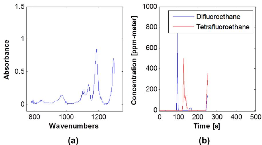
Figure 8: (a) Absorbance spectra at a single moment in time when both difluoroethane and tetrafluoroethane were simultaneously sprayed into the beam path. (b) Gas concentration versus time in units of ppm-meter. The detection algorithm identifies the gas and determines its concentration.
