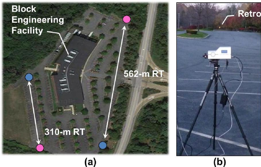
Figure 6: (a) Aerial view of Block's facilities showing the 2 optical paths for testing. (b) Photograph of the tripod-mounted LaserWarn system during the testing. Note the distant retro-reflector which can be seen because a flash was used to take the photograph.
