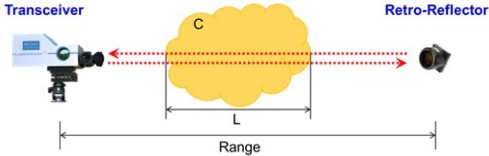
Figure 1: Schematic drawing of open-path atmospheric sensing system that is formed between the laser transceiver and a retro-reflector. Chemical clouds that intercept the laser beam, and that have absorption features within the laser's tuning range, are identified and quantified in terms of their concentration-length (CL) product.
