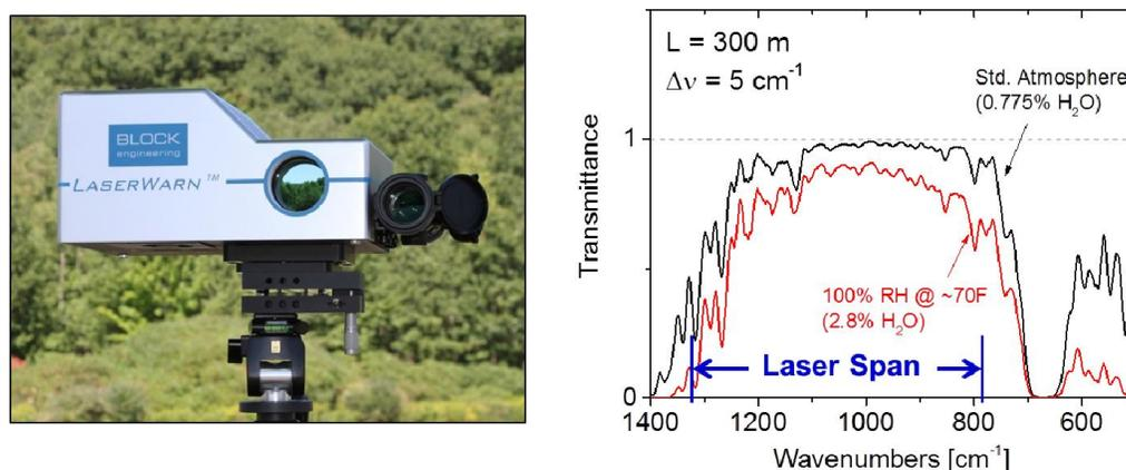
Figure 4: (left) Photograph of the open-path atmospheric sensing system called LaserWarn. (right) LWIR atmospheric transmission window at two humidity levels. Also shown is the spectral range covered by the 2 Mini-QCLs within LaserWarn.
