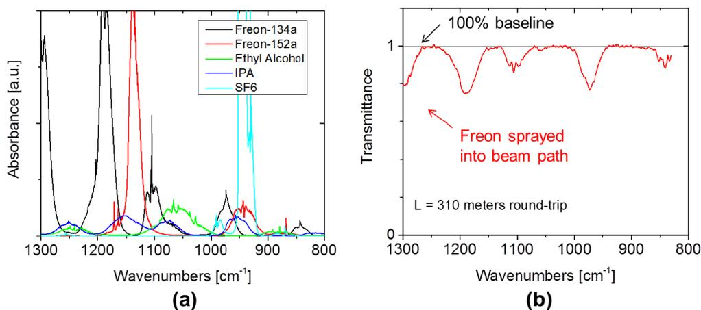
Figure 7: (a) Absorption spectra for various gases that were tested. (b) Transmission spectra when Freon-134a was sprayed into the beam path. The system operated over a 310-m RT path.
