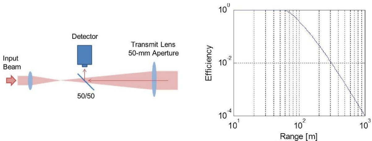
Figure 5: (left) Schematic diagram of the optical design. (right) Optical efficiency versus range when using a 50-mm-diameter retro-reflector.
