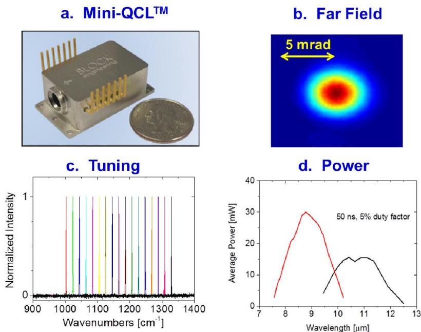
Figure 3: (a) Photograph of a Mini-QCL which is the smallest widely tunable EC-QCL to the best of our knowledge. (b) Image of the far-field beam at  $\lambda = 10 \mu\text{m}$ . (c) Normalized spectra for a Mini-QCL as it is tuned in wavelength. (d) Average power for two different Mini-QCL modules at a duty factor of 5%.
